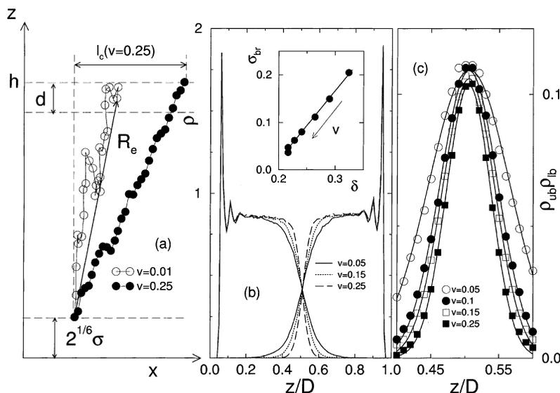
**Figure 2.** (a) Configuration of randomly chosen polymers at two different sliding velocities projected onto the  $(xz)$  plane. (b) Density profile of upper and lower brush. Inset: Shear stress  $\sigma_{br}$  between brushes as a function of overlap distance  $\delta$ . (c) Folded density profile. The lines are fits to the data according to  $\rho_{lb}\rho_{ub} \propto \exp[-(z/D - 0.5)^2/\delta^2]$ , which defines  $\delta$ .
