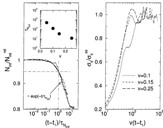
**Figure 10.** Left: Number of interactions as a function of time. The time axis is rescaled so that all data collapse on the same point at unity. Inset: Characteristic time as a function of velocity. Right: Shear stress as a function of driven distance.
