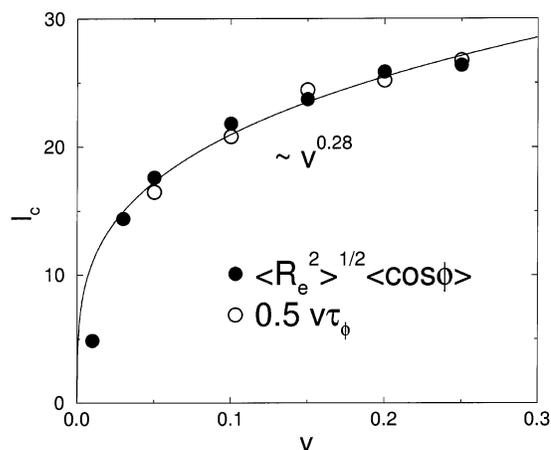
**Figure 5.** Characteristic length  $l_c$  as a function of velocity. Closed points denote the values taken from steady-state examinations, and open symbols refer to our direct measurements of the characteristic times during reverse sliding. The solid line reflects the power law  $v^{0.28}$ .
