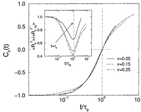
**Figure 6.** Crossover function  $C_c(t)$  defined in eq 6 as a function of normalized time  $t/\tau_\phi$  during stop-and-return for various sliding velocities. Inset: Time dependence of the end-end distance  $R_e$  normalized by the steady-state values.
