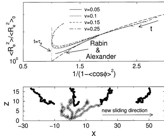
**Figure 7.** Top: Comparison between inclination angle and end-end distance during the transition  $v \rightarrow -v$ . Bottom: Time evolution of a randomly chosen chain from the upper brush (filled symbols) and the lower brush (open symbols) during crossover to a new steady state.
