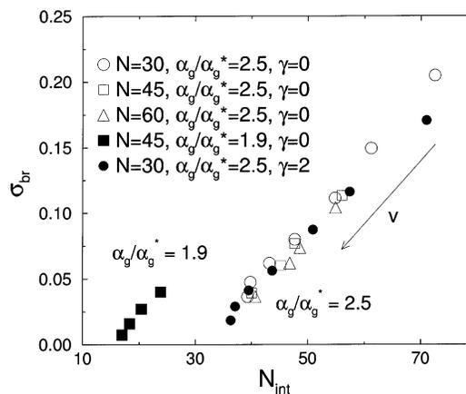
**Figure 3.** Shear stress  $\sigma_{br}$  as a function of brush interdigitation as measured by the number of interactions  $N_{int}$ . Data from previous work, in which the thermostat also acted along the sliding direction ( $\gamma = 2$ ), are included in the figure.
