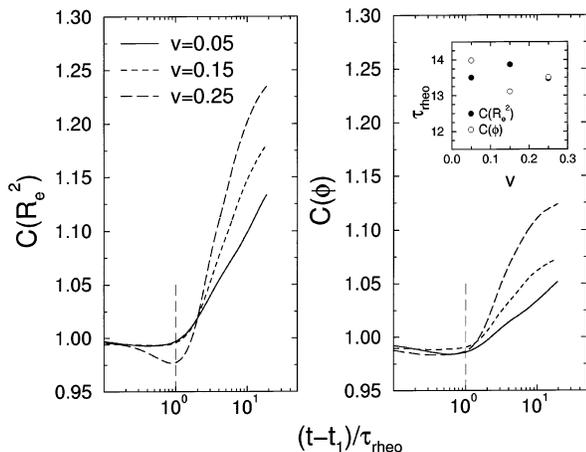
**Figure 9.** Transition functions of rheological observables for the stop-and-go protocol. The time axis is rescaled by the characteristic time  $\tau_{\text{rheo}}$ , defined as the time where  $\partial C(t)/\partial t$  becomes positive. At time  $t = t_1$ , sliding is reinitiated after the system could relax for a time  $t_{\text{rel}} = 50$ . Left: Squared end-to-end distance. Right: Inclination angle. Inset: Characteristic time as a function of velocity.
