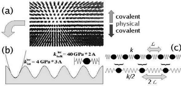
Figure 1. Schematic view of the interaction between two chemically passivated solids.
