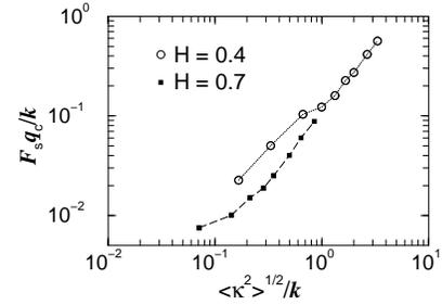
Figure 2. Normalized friction  $F_s q_c / k$  as a function of the normalized, average surface or potential energy curvature  $\sqrt{\langle \kappa^2 \rangle} / k$  for two different Hurst exponents  $H$ .
